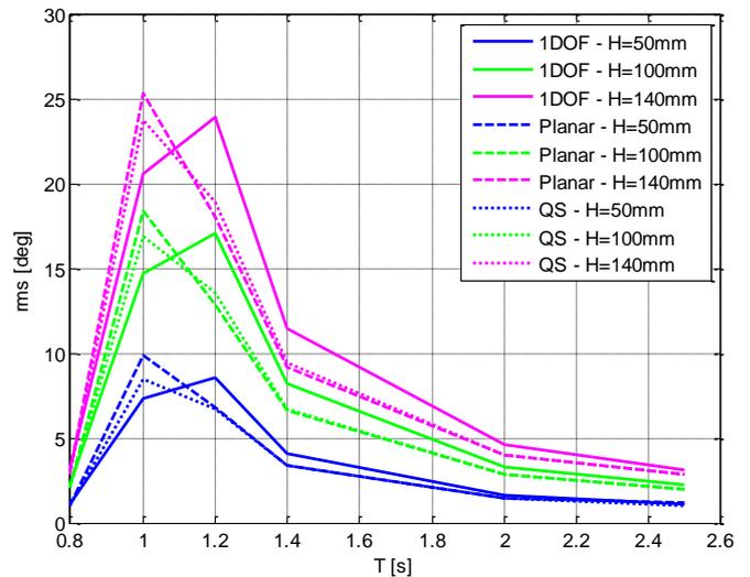
Figure 15. Comparison between steady state rms pitch values, pitch DOF model, ISWEC planar model coupled with quasi-static model and ISWEC planar model coupled with MoorDyn.
