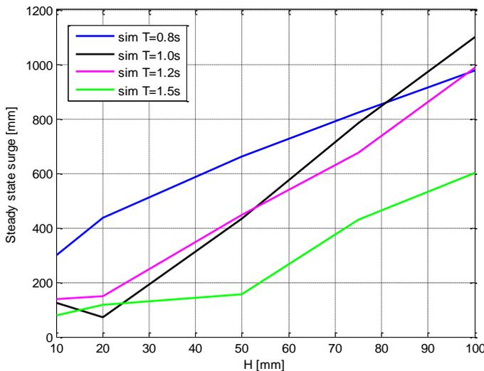
Figure 14. Simulink model coupled with MoorDyn. Surge steady state curves.
