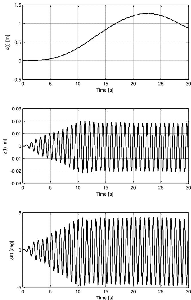
Figure 16. Time history results. Excitation wave: period 0.8 s height 75 mm. The first transient is shown.
