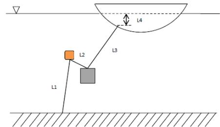
Figure 2. ISWEC mooring system concept
