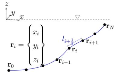
Figure 5. Mooring discretization and indexing
