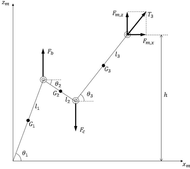
Figure 3. Quasi-static model scheme
