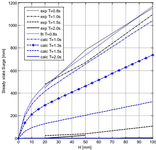
Figure 13. Comparison between experimental and calculated steady state surge curves
