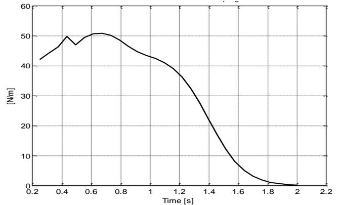
Figure 12. ISWEC 1to20 surge damping coefficient. Evaluated with Ansys AQWA.
