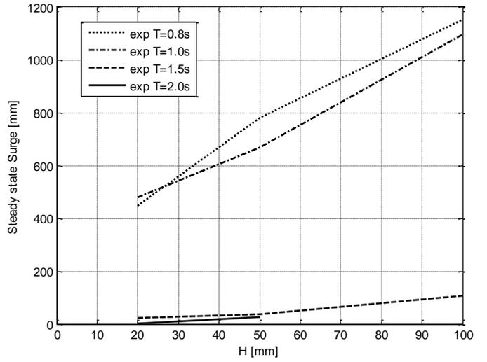
Figure 11 . Experimental data, ISWEC 1:20 scale model. Steady state surge position in function of wave height H and wave period T.
