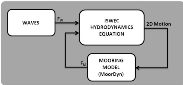
Figure 8. ISWEC hydrodynamic expanded model functional diagram.
