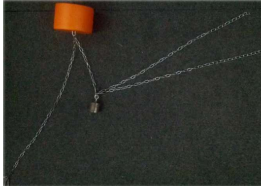
Figure 2.20: Mooring system used in 1:20-scale ISWEC tests (image courtesy of Giacomo Vissio)
