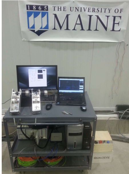
Figure 6.1: Hybrid coupling system used at basin
