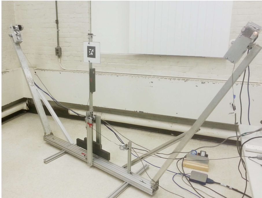
Figure 5.5: Test rig with opposing winch units and 1:100-scale pendulum
