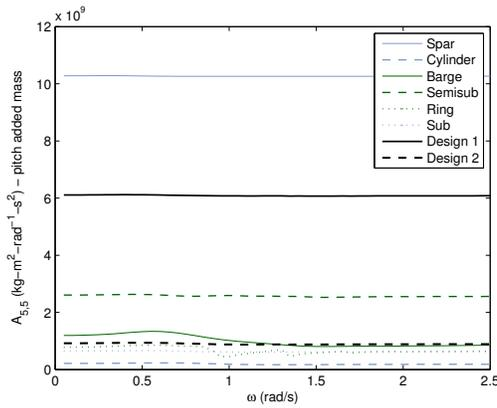
Figure 4.5: Pitch added mass for catenary-moored platforms
