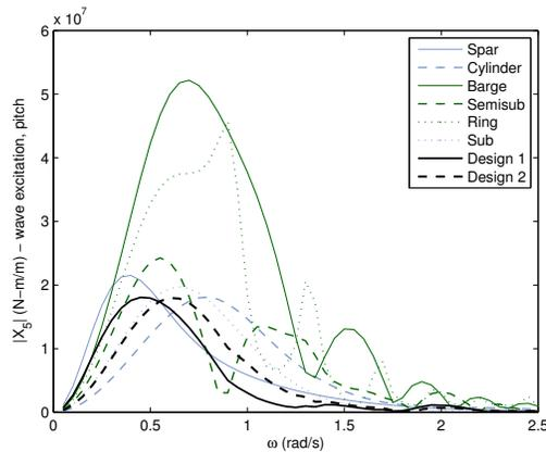
Figure 4.7: Pitch wave excitation for catenary-moored platforms
