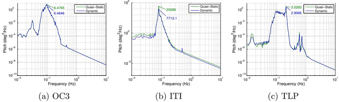
Figure 3.7: LC 4.2 - platform pitch PSD
