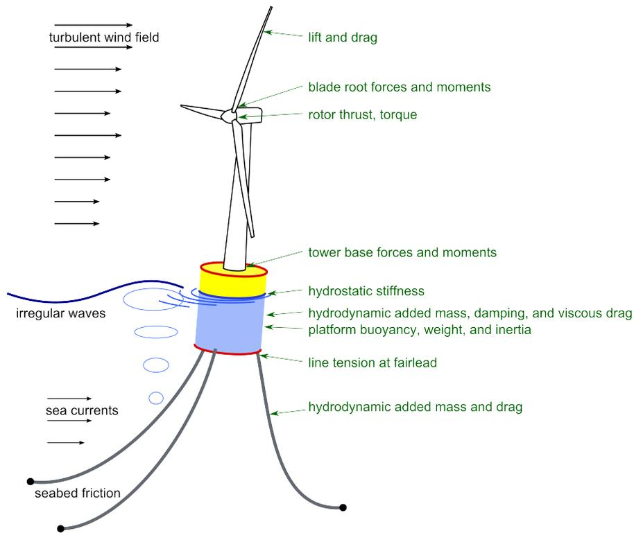
Figure 2.1: Important loads on a floating wind turbine
