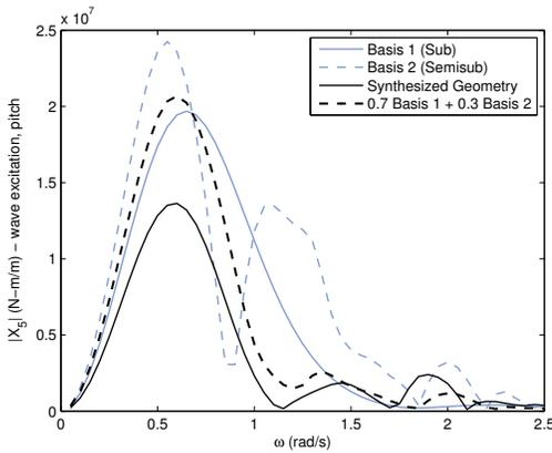
Figure 4.20: Pitch wave excitation of combined platforms
