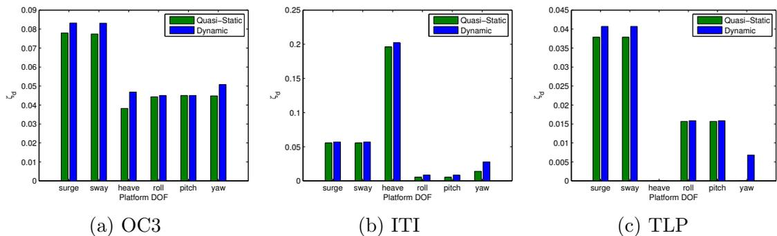
Figure 3.4: LC 1.4 - platform damping ratios
