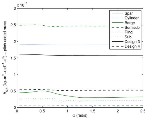
Figure 4.10: Pitch added mass for tension-leg-moored platforms
