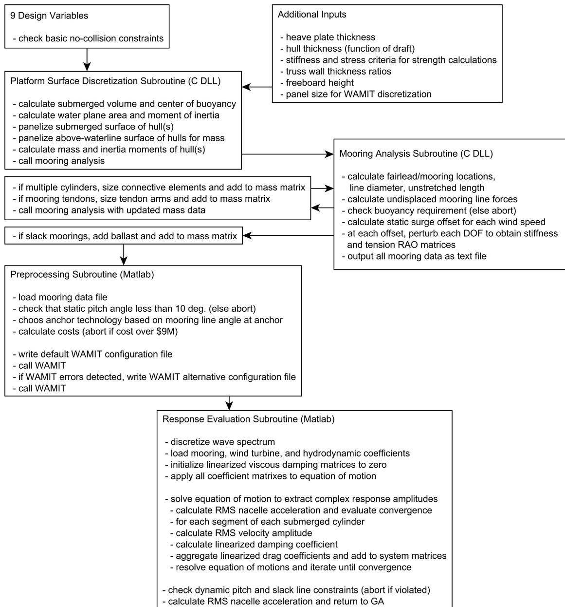
Figure 5.8: Flow diagram of design evaluation implementation
