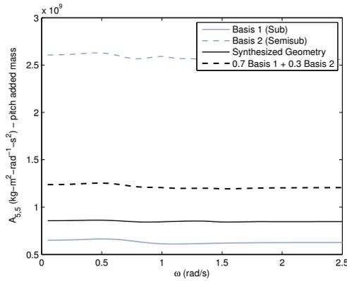
Figure 4.18: Pitch added mass of combined platforms
