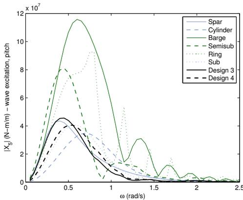
Figure 4.12: Pitch wave excitation for tension-leg-moored platforms
