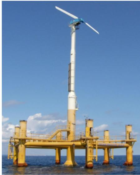
Figure 1.3: The Blue H 80 kW mooring-stabilized prototype
